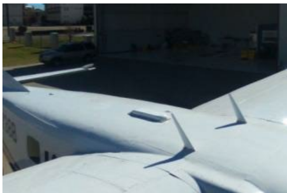
FIGURE 26 - Satellite Communication System Phased Array Antenna
